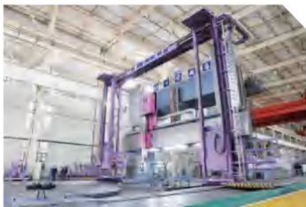
XKA28105×300 数控重型桥式龙门五轴联动车铣复合机床
