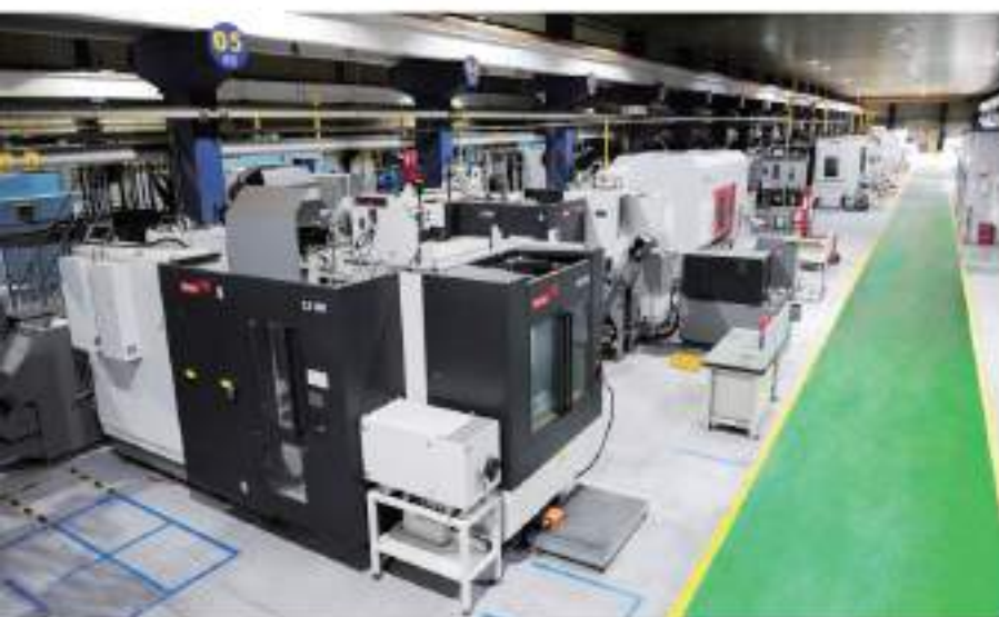
先进的制造加工设备：叶片加工数控机床 Advanced manufacturing and processing equipment: CNC machine tools for blade processing
